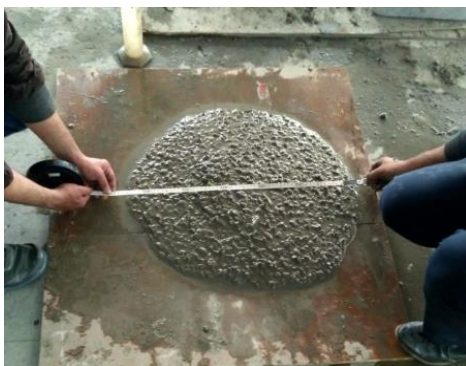
Fig. 2. Slump Test for SCC
