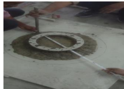
Fig. 3. J-Ring test for SCC
