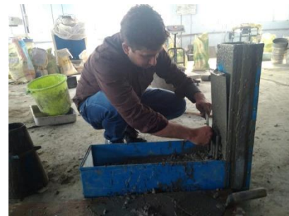
Fig. 5. L-box test for SCC
